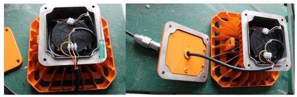
4) Put the driver cover back and tighten the 4 screws.
